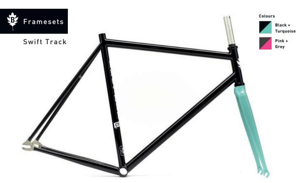
Our infamous Swift track frame is back again in 2016. Featuring double oversize tig welded tubing, carbon forks and our custom Brother polished stainless steel track dropouts. The aggressive track geometry gives the Swift a nimble and responsive ride making it an effective race bike on the street or track. The 2016 model now comes with colour clash pink or turquoise forks, all black forks are also available for a stealth look.
